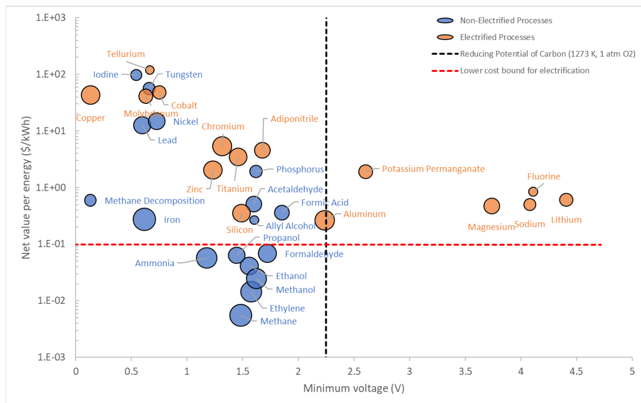
Figure 7. Commodity chemicals produced by oxidation/reduction. Orange points involve pure thermal unit operations, and blue points indicate processes that are conducted electrochemically to any appreciable extent in industry. The horizontal red line represents the empirical lower bound of feasibility for electrification in terms of dollars of product per kWh of energy used while the vertical black line represents the practical maximum reduction potential of carbon at 1000 °C. Marker sizes indicate the market volume of each commodity in tons/yr.
